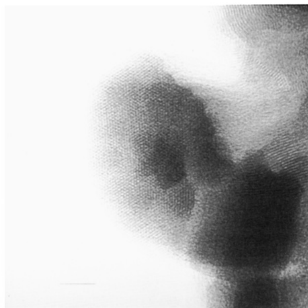
Figure 5. (a, top) TEM image showing parallel lines and honeycomb-like structure arising from channels and their extremities respectively (bar = 50 nm). (b, bottom) Lines have disappeared after slight tilt around the axis of channels (bar = 50 nm).
